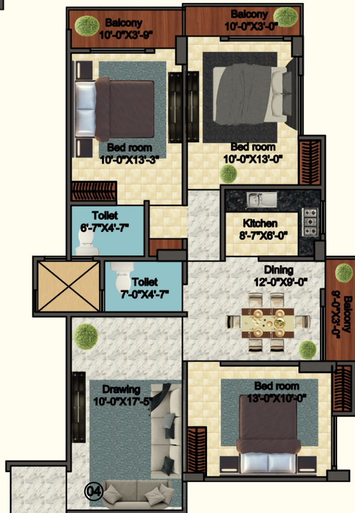
4 IRIS 1442 3 BHK + 2 TOILETS + 3 Balcony Balcony Area : 98 Sq. Ft. B/U Area : 1030Sq. Ft.
